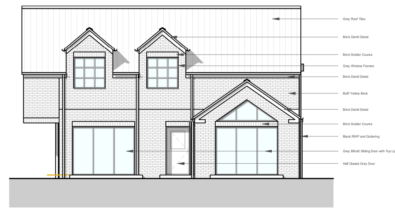
General Arrangement - Rear Elevation 1 : 100
