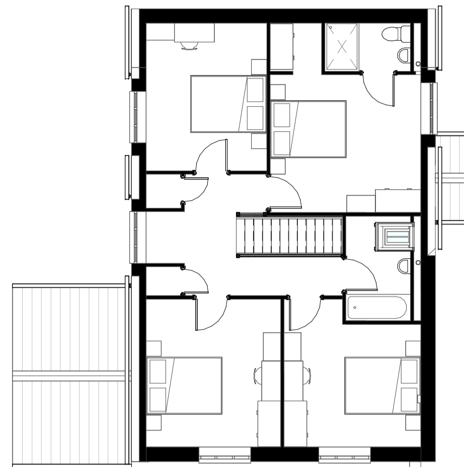
General Arrangement - First Floor 1 : 100
