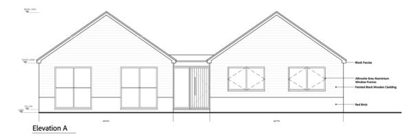
The external walls will be constructed of low-level red brick, with black timber cladding to the eaves. Red/brown tiles are proposed for the roof.
